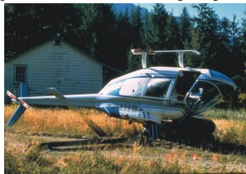
The cause was easy to find when the engine cowls were opened, for there on the deck lay the N1 cannon plug. The AME/AMT was absolutely sure he had tightened the plug on the tach generator but had no explanation for how it could have come
